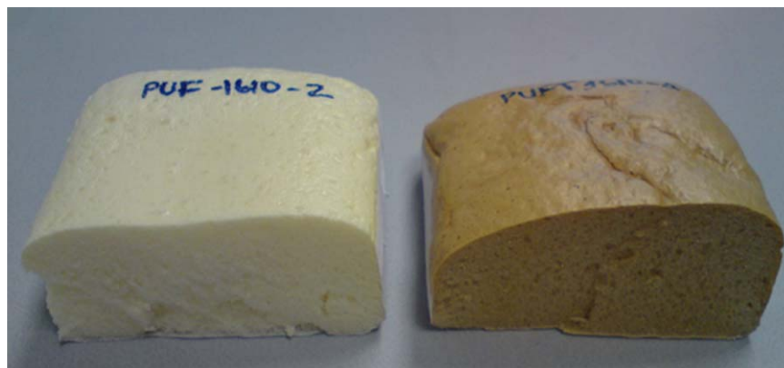
Figure 5. PU foams synthesized from HTPI (left) and from HTO (right). [Color figure can be viewed in the online issue, which is available at wileyonlinelibrary.com .]
